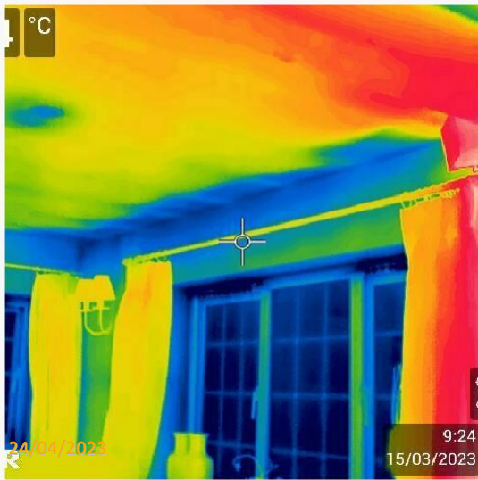
Thermogram showing heat loss through eaves Photo detail
