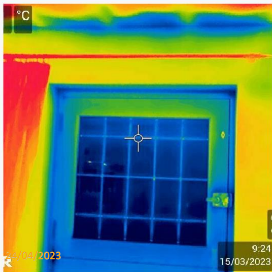
Thermogram showing draughts and heat loss through rear door
