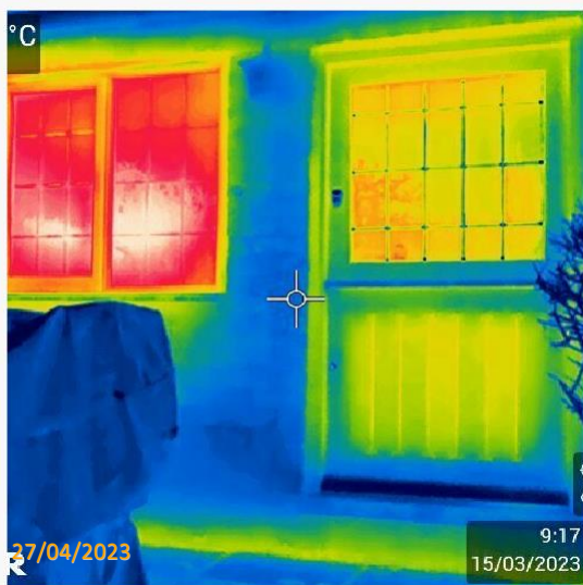
Heat loss noted to lower door
